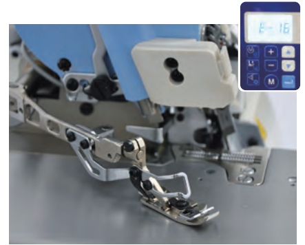
3. Presser foot arm with an open/close sensor
